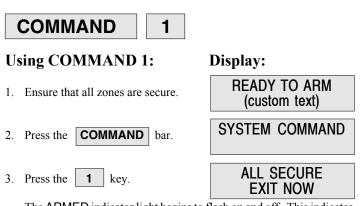
The **ARMED** indicator light begins to flash on and off. This indicates that the system has begun exit delay time.
