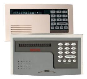
Each D1255 Series VFD Keypad model is an SDI bus compatible device that works with the G Series Control Panels and the D9124 Addressable Fire Alarm Panel. Each keypad model has an illuminated keypad, 16character English language vacuum fluorescent display (VFD), and a sounder that emits eight tones.
